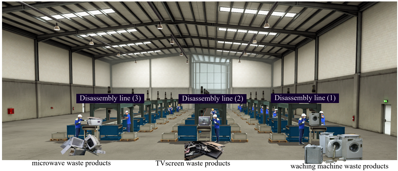
Fig. 1. Traditional parallel layout disassembly line dividing to three lines, every line assigned to one type of waste product.
