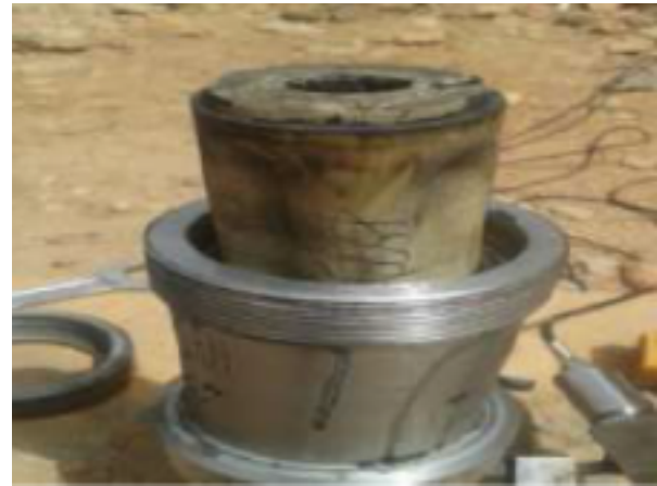
Fig. 6. Insulator after test in real product
