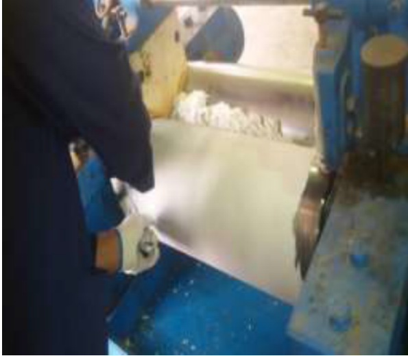
Fig. 3. Producing the insulator sheet using rolling machine.
