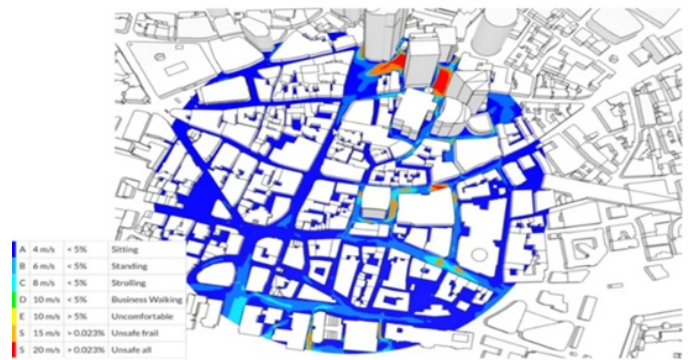
Pedestrian wind comfort simulation of Central London
